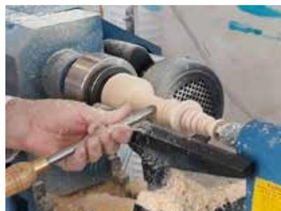
**The final king being turned on the lathe.**
