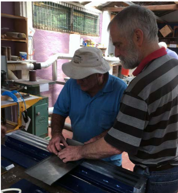
Learning to use the new sheet-metal bender.
