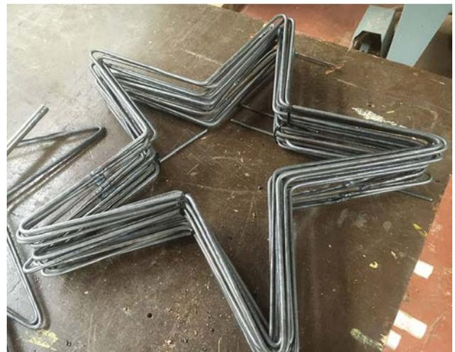
**A bundle of 20 completed stars. Each star is bent to shape on Joe's jig, then the ends are welded together.**
