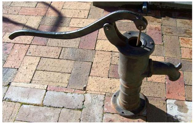
**The hand water pump after cleaning, oiling and reassembly.**
